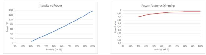
Power consumption versus dimming ratio and power factor (PF) vs dimming
