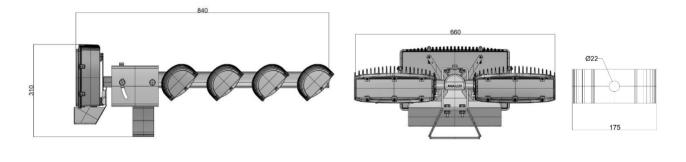
CE marking is applicable Gland dimensions incoming supply voltage wire: M25 Cable diameter acceptance 10 – 14mm Underslung mounting possible – see manual
